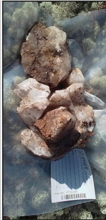
Rusted quartz vein (right) collected from weakly altered metasedimentary rocks (above) returned an assay of 0.272 g/t gold.
